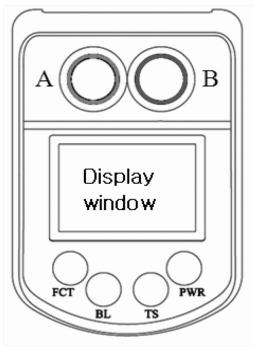
A: Cuvette holder for protein measurement 蛋白質測量處
