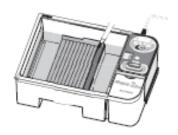
2) After verifying that the operation switch of the power supply is OFF, close the migration tank lid.
