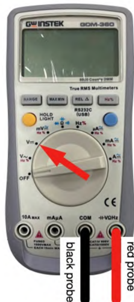
Figure P-3. shows the multimeter used in this exam together with location of the probes and the mode selection.
